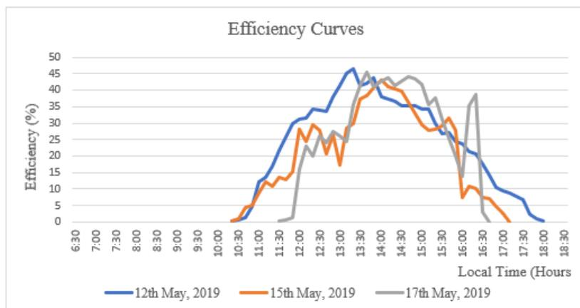
Fig. 2. Instantaneous thermal efficiency curves as a function of time of the Day for 12<sup>th</sup>, 15<sup>th</sup> and 17<sup>th</sup> May 2019
