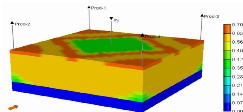
Fig. 4. Steam flooding in an inverted 5-spot grid (CNPC, 2011)
