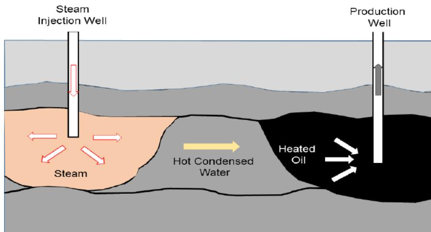
Fig. 3. Mechanism of steam flooding process (Wei Z, 2016)
